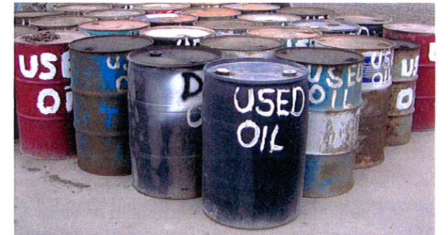
Simple labels on containers can satisfy used oil labeling requirements. Label used oil containers with the words "Used Oil."
