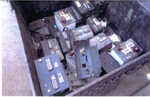
Lead-acid batteries should be stored in closed, plastic containers. The storage area should be protected from weather and be designed so that any accidental spill does not reach a pervious surface.
